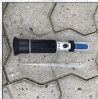
Refractometer and pipette for checking mixing ratio
