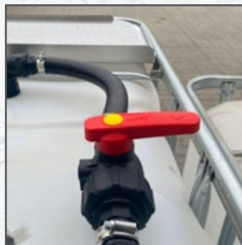
Three-way valve with two settings
